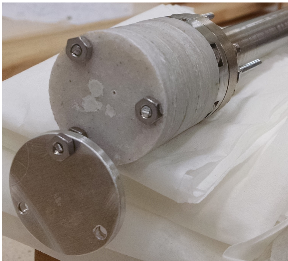
Figure 5. A photograph of the Mochi.GEA with the pinhole aperture and gate installed. The other three holes filled in with Torr Seal® are visible as well.
