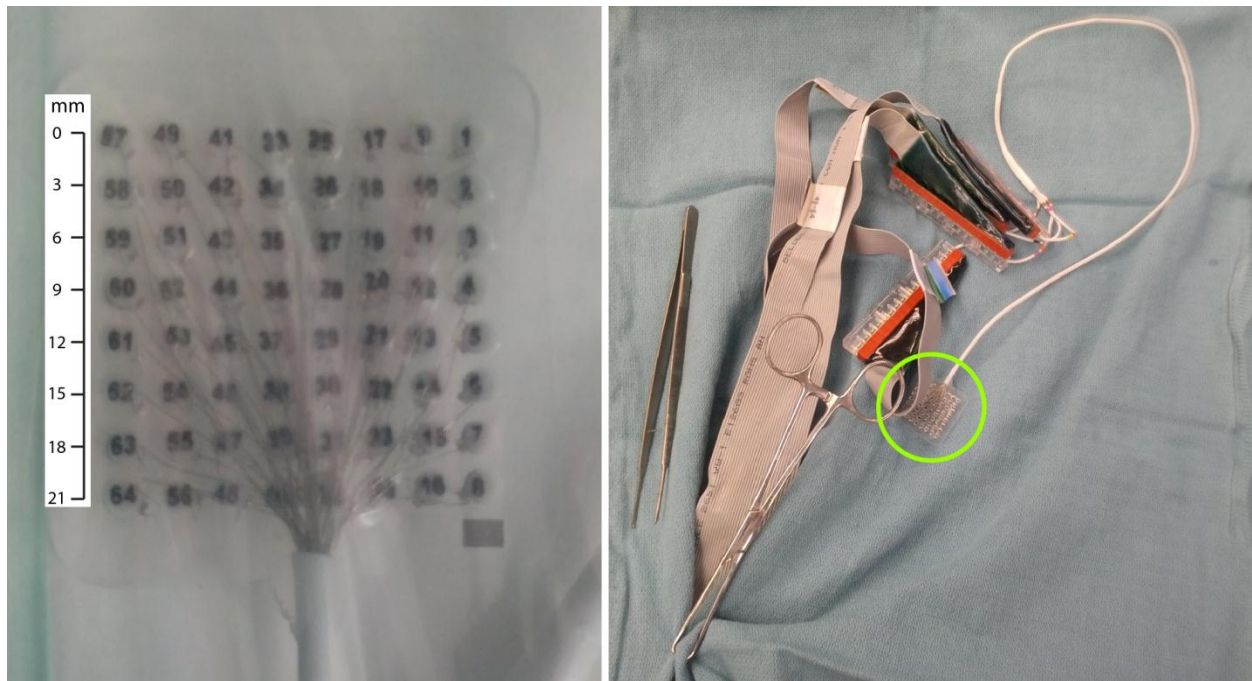
Figure 30 – Image of the microgrid that was implanted. It's scale can be seen next to a set of standard clinical forceps. All 64 contacts come out in a single wire that splits in to four 16-contact pig-tails. Each pigtail was plugged into a single biosignal amplifier.
