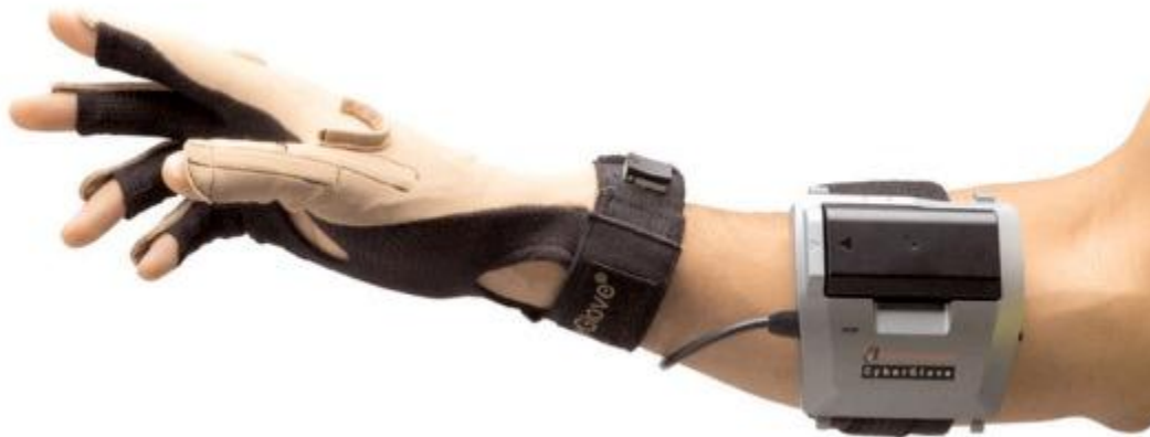
Figure 18 – CybergloveII dataglove used to record joint angles
