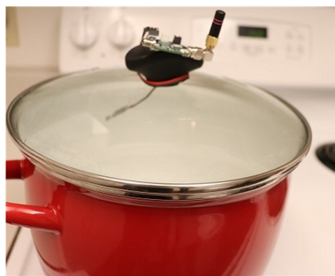
(a) Pot with temperature sensor and BLE tag.
