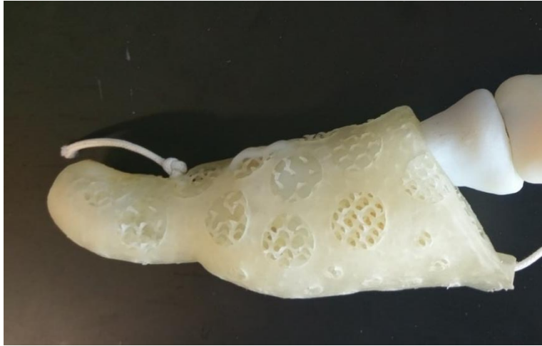
Figure 3.7. First ray BAREFOOT model with gyroid lattice microstructure.
