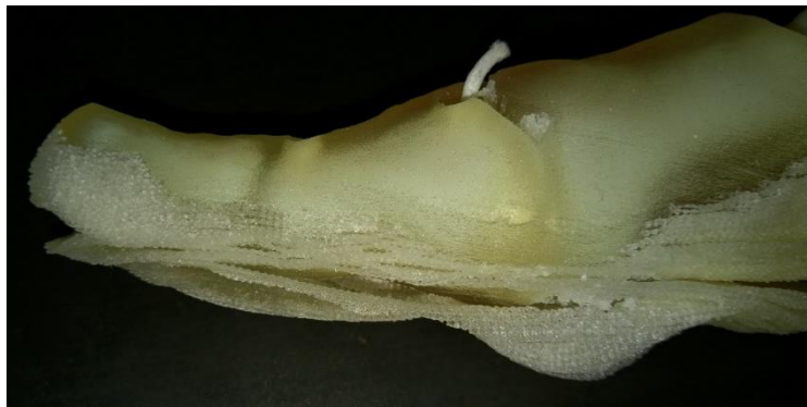
Figure 3.5. Cubic lattice applied to first ray BAREFOOT model. Peeling along layers was an issue and was the primary motivation to seek a new lattice type.
