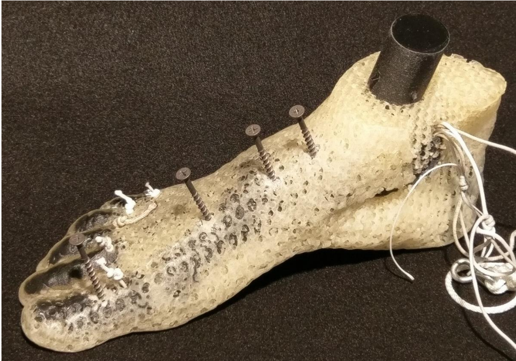
Figure 4.4. Photo of printed BAREFOOT model after support dissolution and tendon routing, ready to be tested on the RGS.
