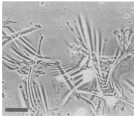
Figure 3. Silicone rubber membrane wrinkles due to the traction forces from several chick heart fibroblasts. Reproduced from (22). Bar: 100 \mu\text{m} .
