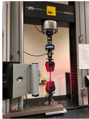
Figure 20. Tensile test with DIC setup
