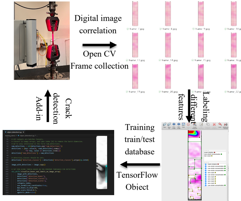
Figure 28. Process of crack detection by CNN
