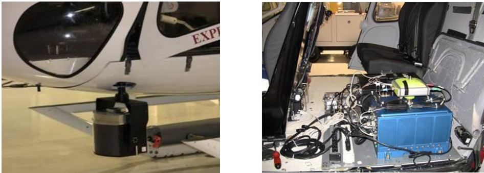
Figure 2.2 The front-end and back-end unit of the active millimeter-wave radar system.
