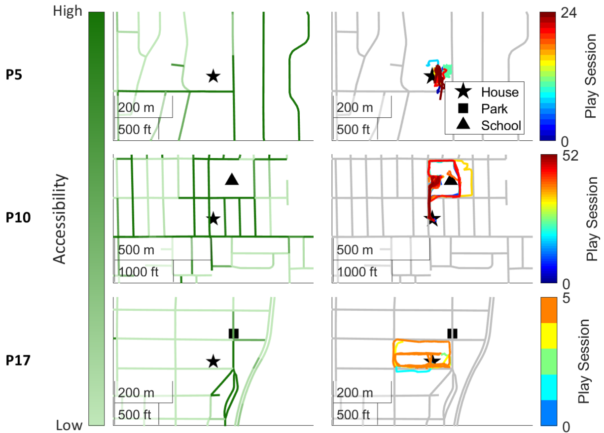
Figure 3.8: The accessibility scores for the sidewalks near each participant’s (P5, P10, P17) home on the left and the drive path of the participant on the right. Participants generally avoided driving on streets that were not accessible.
