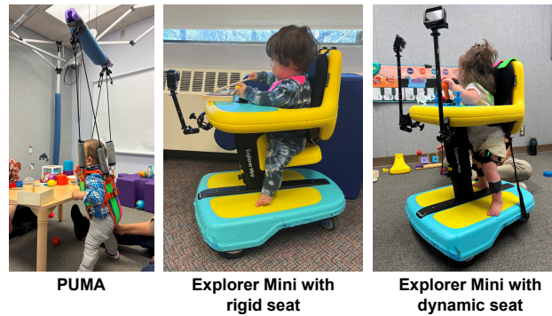
Figure 7.1: The Portable Mobility Aid for Children (PUMA) and the Permobil Explorer Mini using the rigid seat and dynamic seat configurations.
