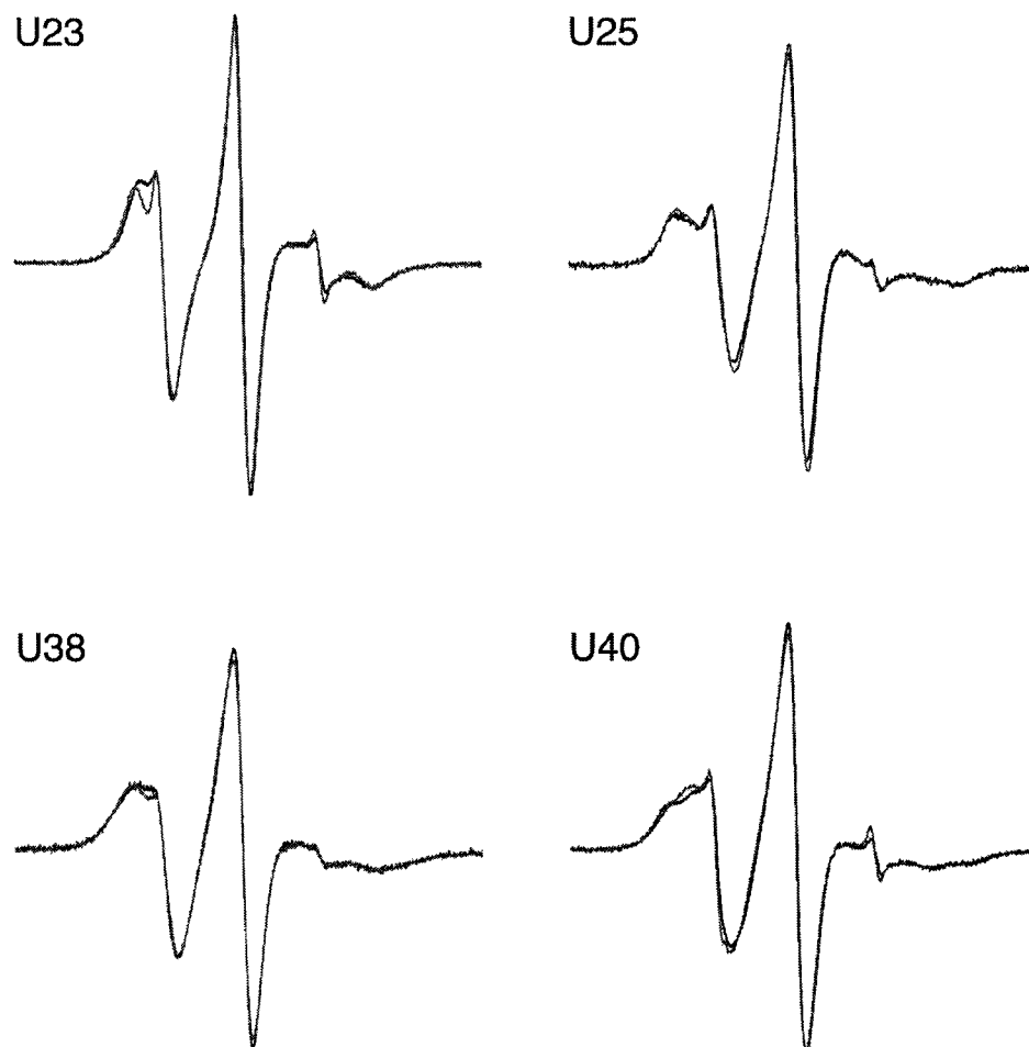
Figure 8.14. EPR spectra of spin-labeled TAR RNAs in the absence (black) and presence (gray) of 30 mM SrCl 2 in 20% sucrose/1.0 mM potassium phosphate, pH 6.5.
