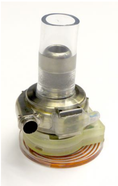
Figure 3.35: FREE-D receiver and Rx coil mounted on HeartWare HVAD.
