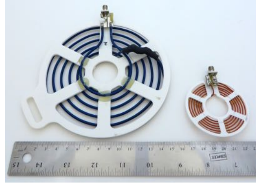
Figure 3.10: Front side of Tx and Rx coils used for the FREE-D system. Figure 3.11: Back side of Tx and Rx coils used for the FREE-D System.
