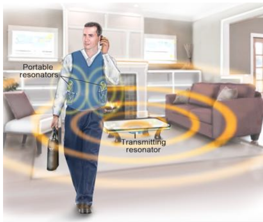
Figure 3.3: Long-range FREE-D system with transmit resonators installed throughout the patient's home.
