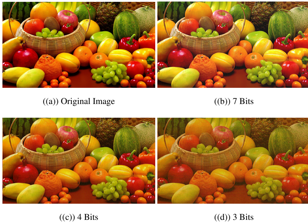
Figure 2.10: Effective Number of Bits (ENOB) versus video quality. The frame corresponding to an ENOB of 3 (d) shows video quality degradation.
