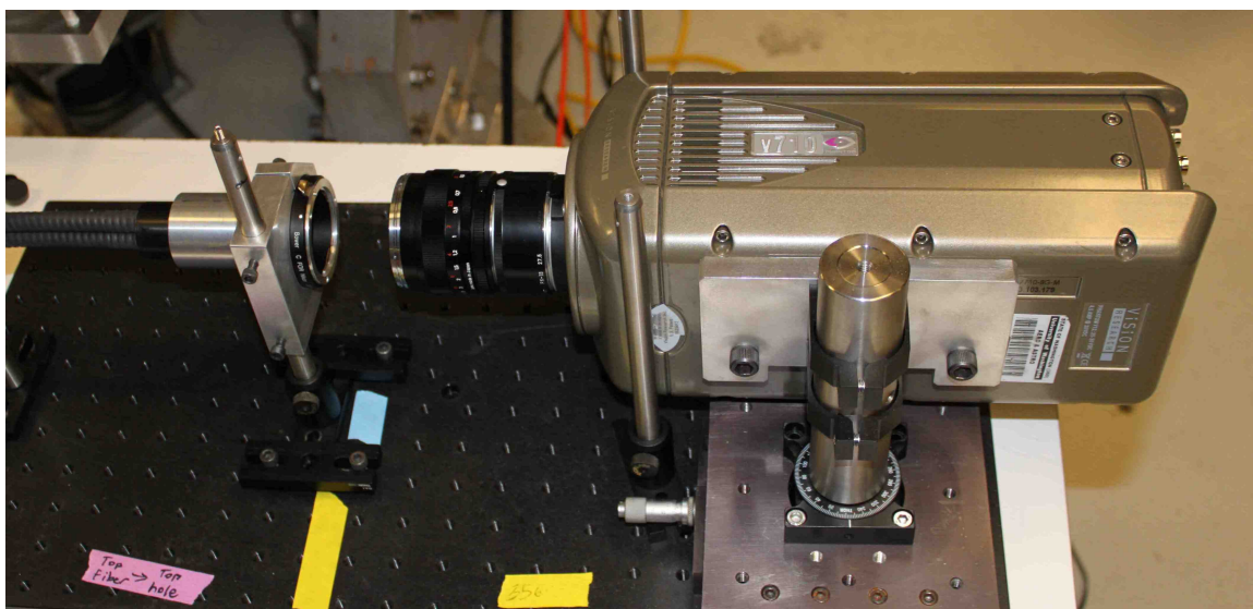
Figure 5.28: The high-speed camera images the output of both coherent fibers simultaneously.
