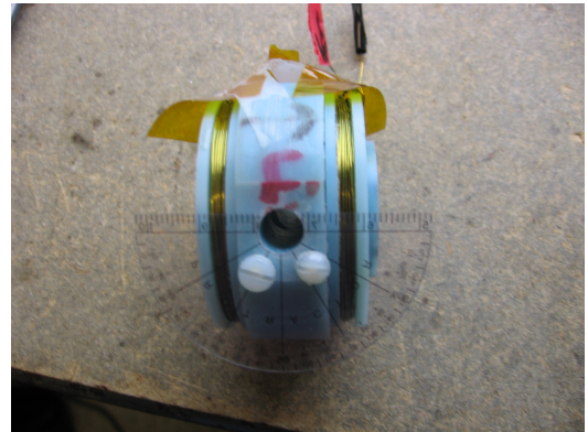
Figure 5.11: Orientation of the Helmholtz coil used for the calibration of the transverse pickup coils. Coil designed by R. J. Smith.
