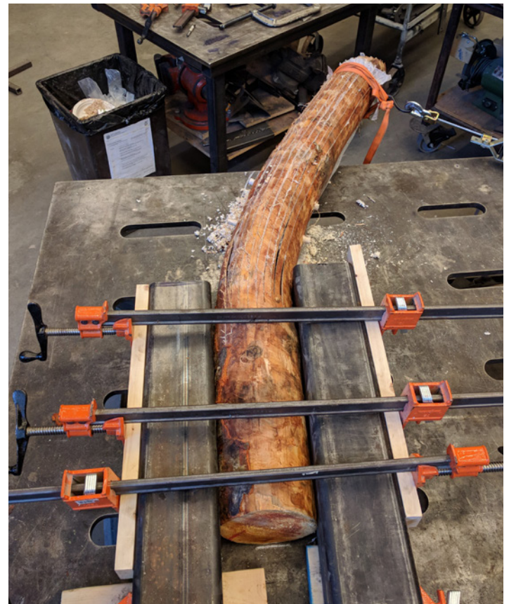
Figure 36. Bending sliced log with 2,000lb come-a-long 1
