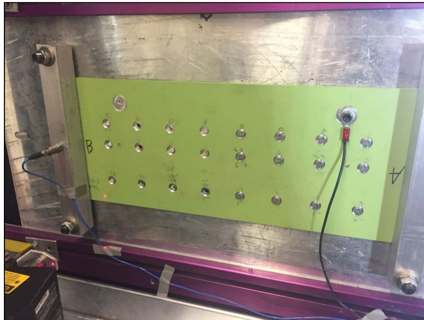
Figure 3.1: Mounted coupon with short edges clamped
