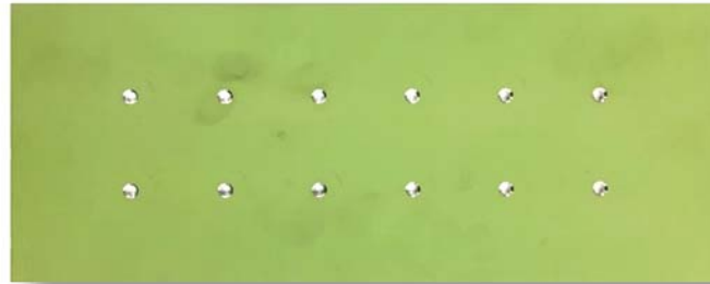
Figure 1.1: Example of surrogate coupon used in riveting tests to evaluate tool effectiveness.
