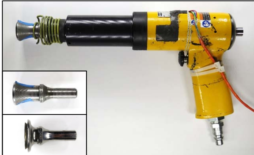
Figure 4.1: Atlas Copco RRH 10P TS rivet gun with .33 lb. hammer (top) and .287 lb. hammer (bottom)
