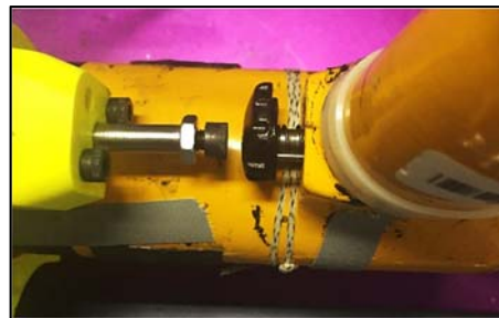
Figure 4.2: Rivet gun trigger setting, with firing mechanism
