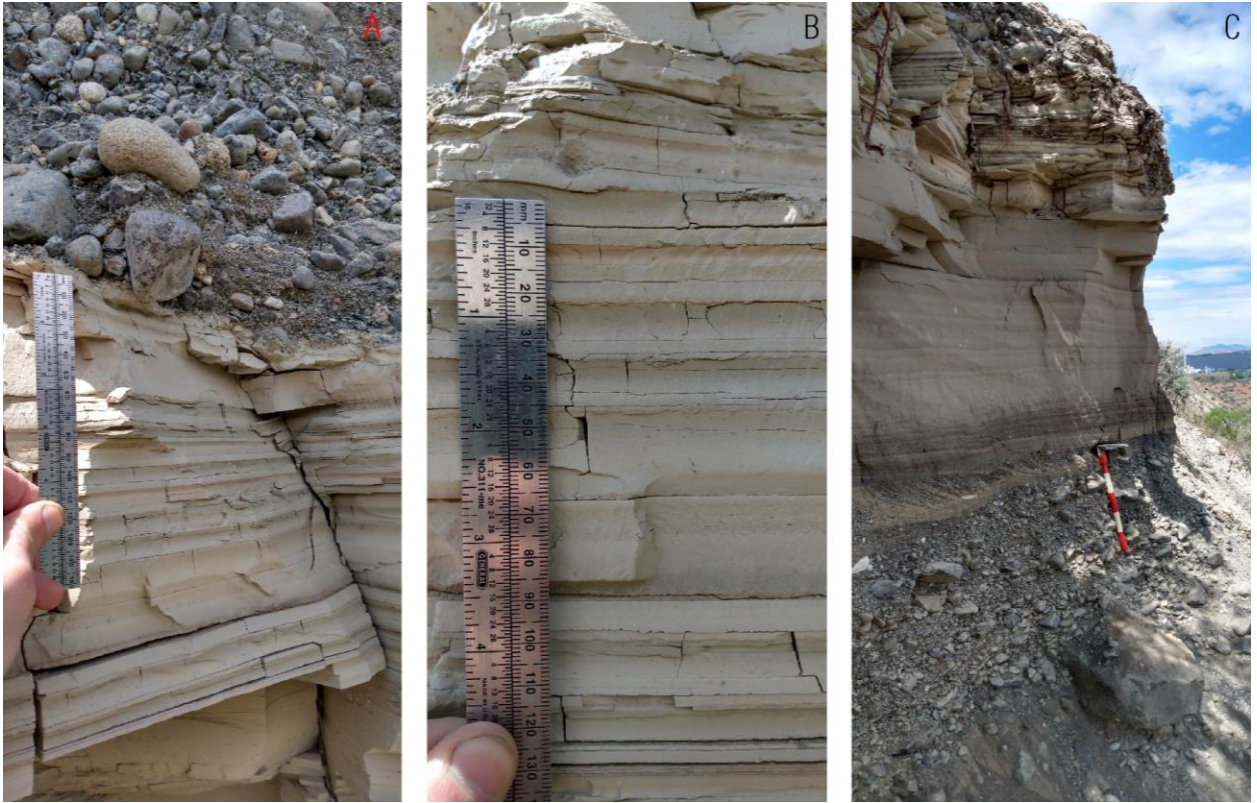
Figure 3-12: Varves of Rock Island delta. (A) Erosive contact between cobble gravel and varves. (B) Details of varves above gravel near top of section (C) Typical fining upward sequence of cobble gravel to silt transitioning into varves.
