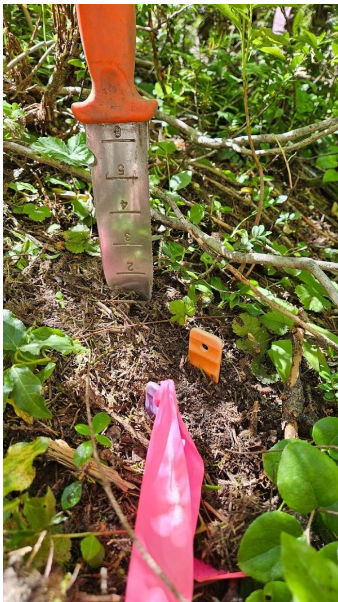
Figure 10. Cation (purple with pink flagging) and anion soil probes (orange) used to quantify soil nutrients at plots on the Gifford Pinchot National Forest, Washington, USA (cf. Table 2).
