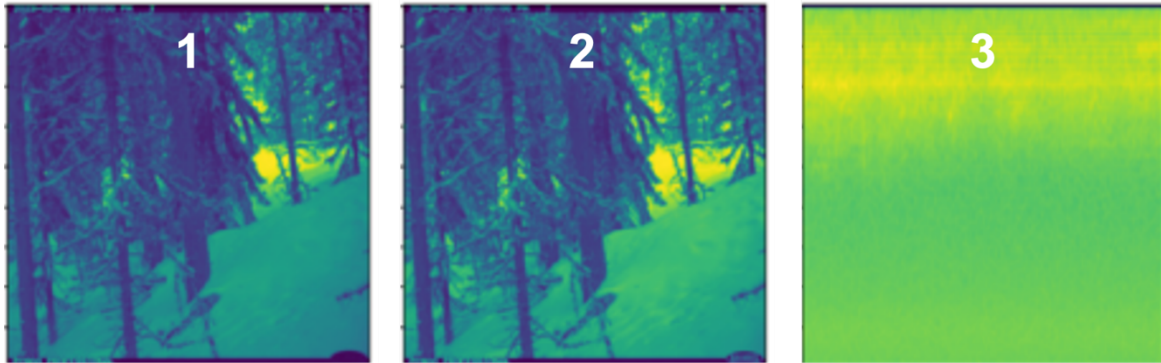
Figure 6.2 Example input data for our image+audio model. The ResNet-50 model architecture requires input data to have 3 channels, so we used the first two channels for the red and green channels of the RGB camera image, and for the third channel, we used the spectrograph from the AudioMoth recording.
