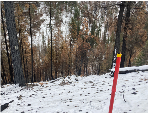
Figure B2. A) Example set-up on Grand Mesa, Colorado. Wingscape cameras (WCT-00126 TimeLapseCam Pro) were installed on t-post driven into the ground. B) Example set-up in Okanogan County, Washington. Reconyx cameras were set up on trees using a cable lock to secure the camera in place.
