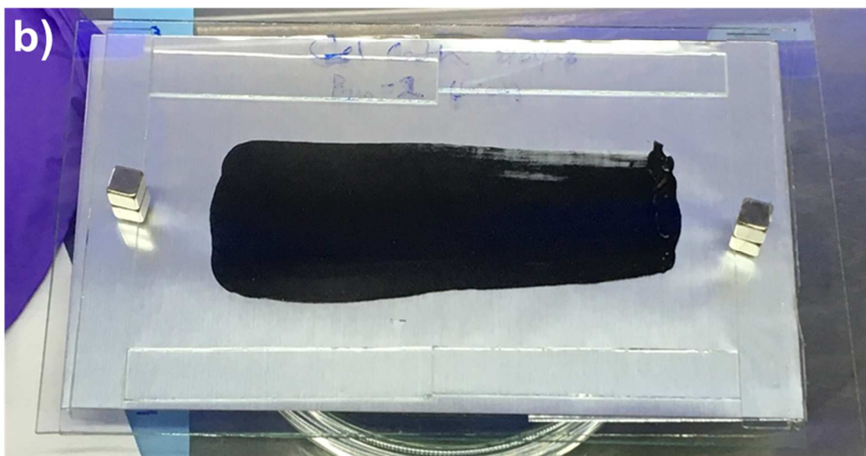
Figure 5.5. a) Schematic of the fabrication process for C/S/SIG composite cathodes. b) Image of a cured C/S/SIG film. This early trial used glass spacers, which were later replaced by an EPDM rubber spacer.
