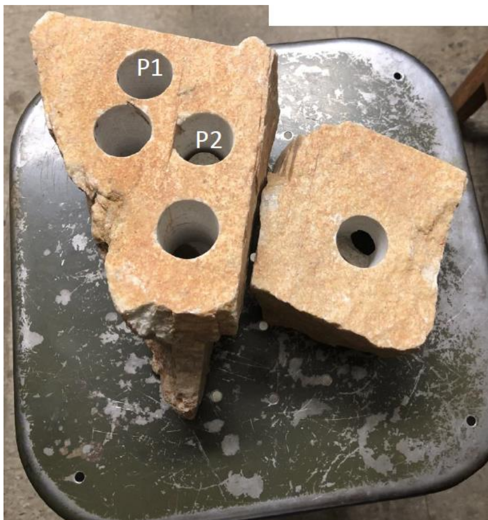
Samples acquired from rock P – rock was cut into two pieces to accommodate the core drilling instrument used acquire some samples.
