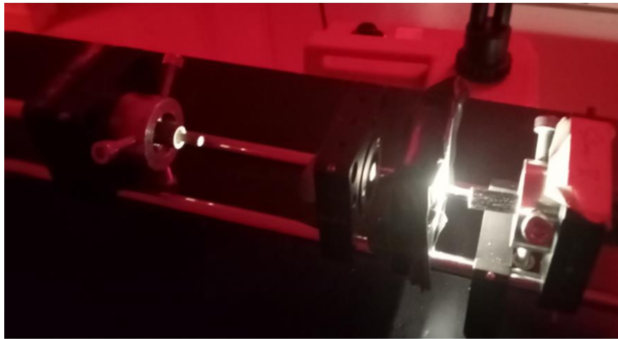
Spectrometer (left) lined up to light source (right). Near the light source are the two 1 mm light filters used to direct incident light onto sample.
