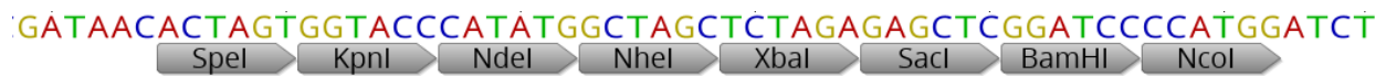
Figure 2.2 HaloTag multicloning site map. Constructed multi-cloning site for HaloTag constructs with 18AA spacer between HaloTag and antigen of interest.
