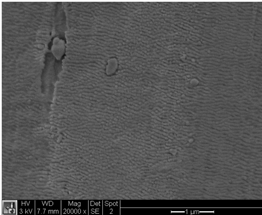
Figure 82. Electron micrograph of atmospheric pressure plasma treated PFG 52006 nylon peel ply at (a) 10,000X and (b) 20,000X.
