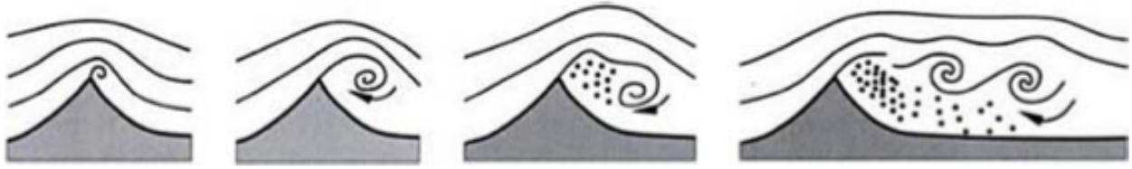
Figure 53. Schematic of vorticity suggesting why atmospheric pressure plasma may not directly interact with the surface within the peel ply channels. [31]
