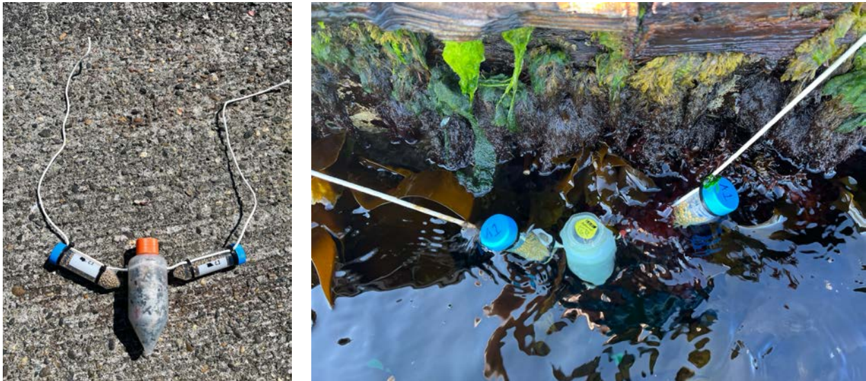
Figure 1. a) Falcon tubes ziptied to cotton rope, with a weight in between the falcon tubes. b) The falcon tubes and weight hanging from the cotton rope, secured to the dock.
