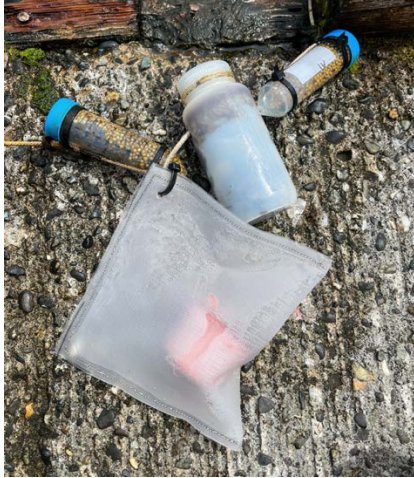
Figure 2. Carbaryl plaster block in a mesh bag, next to the weight so that it remains submerged.
