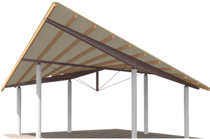
Fig. 5.28: A conventional framing plan for a hyperbolic paraboloid roof follows common rules of beam hierarchy.
