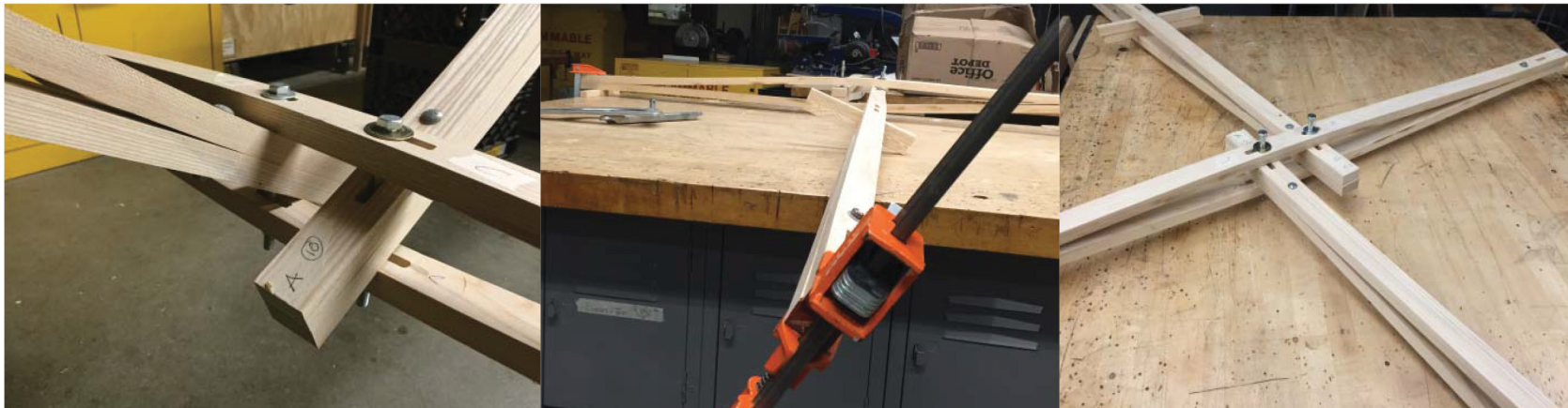
Fig. 5.10: Requirements for joint performance are extracted from the model. Rotational freedoms provided by the slot length perform as designed, and the material appears capable of handling the necessary torque and flex without any sign of failure.
