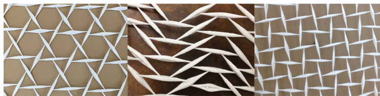
Fig. 5.30: Pattern and topology variation may add lateral stability.
