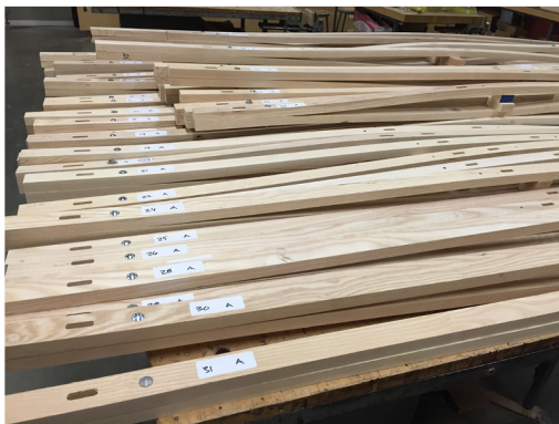
Fig. 5.19: Pre-fabrication is carried out using simple documentation. The form of the installation is coded in this length data, but not apparent until assembly.
