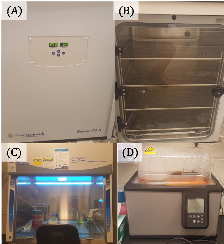
Figure 2.12. Images showing key instruments required for cell culture process: (A) incubator showing the temperature and carbon content, (B) incubator shelf, (C) bio-hood facility equipped with UV cleaning system, and (D) hot bath for thawing process.
