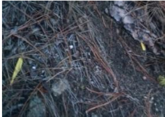
Figure A.3(Right) 6 months following the application of fluorescent mineral particles at Site 2, approximately 30-40% of the particles were observed. The majority of mineral particles remaining were between 2-5 mm (the intermediate size class of the applied minerals). Erosion pins are marked with yellow flagging.
