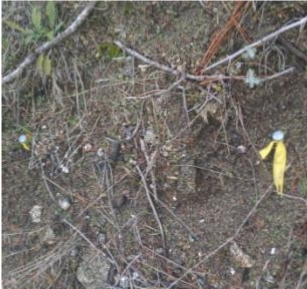
Figure A.2(Left) Erosion pins installed at Site 1 which has a slope of 38 degrees. Pins were marked with flagging to aid in recovery upon revisits. 6 months following the application of the fluorescent mineral particles, approximately 40-50% of the particles remained. Erosion pins are marked with yellow flagging.
