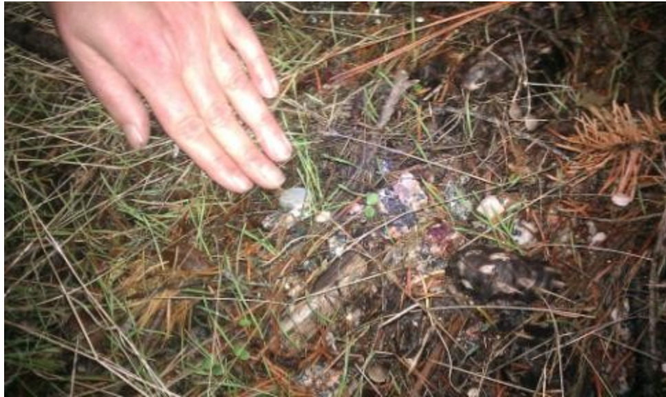
Figure A.5 (top) Willemite particles distributed between erosion pins at Site 3. This location was had a significant accumulation of organic matter relative to the other sites and was situated on a relatively flat shelf of the slope. (bottom) Willemite particles distributed between erosion pins at site 3 fluorescing beneath the application of ultra violet. Willemite fluoresces to green and calcite can be seen as the red fluorescence
