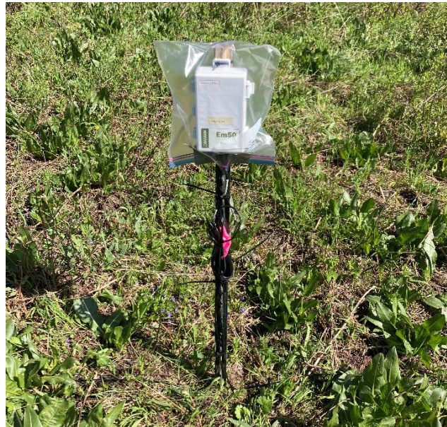
Figure 2.3 Data logger affixed to t-post with sensors installed.
