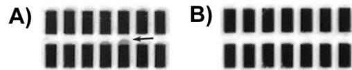
Figure 3.9. Images of filled chambers at ambient pressure following sample digitization. A) When using an air compressor to drive flow during digitization, some chambers overflow and sample is pushed into the main channel after pressure is released. The arrow indicates an area where sample exits the chamber. B) When vacuum pressure was used to digitize the sample this effect was not present.
