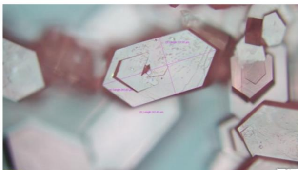
Figure 18 shows the Marimuthu et al.'s synthesized cobalt formate crystals with a white scale bar of 50 um.
