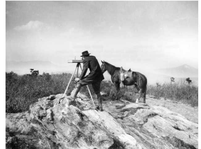
Figure 6: Sighting a fire using a portable firefinder, 1916.
