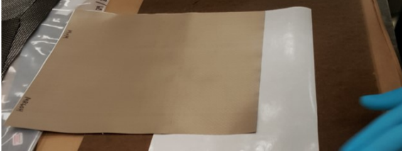
Figure 21: Cutting resin film to panel length for prepregging dry fiber plain weave panels with epoxy resin
