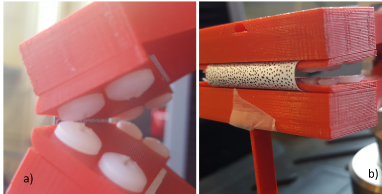
Figure 37: Limitations of fixtures when small grip separations are required: a) v6 screws are interfering and b) v7 has enough clearance
