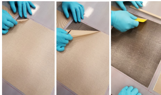
Figure 23: Manual laying up prepregged HTA40 PW for CPW panel
