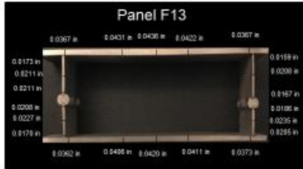
Figure 5.8 - Sample panel measurements with the thickness values and line locations of measure distances
