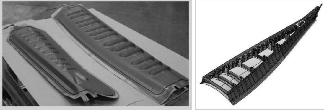
Figure 2.11 - Two sheet SPF/DB at Boeing [9]
