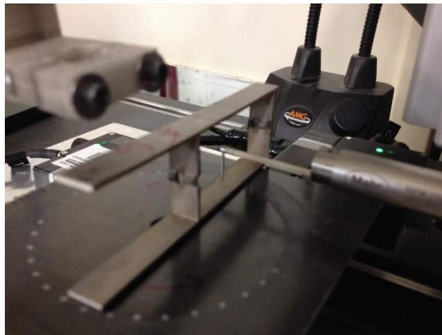
Figure 7.7 - Surface profile location when testing the roughening during superplasticity.
