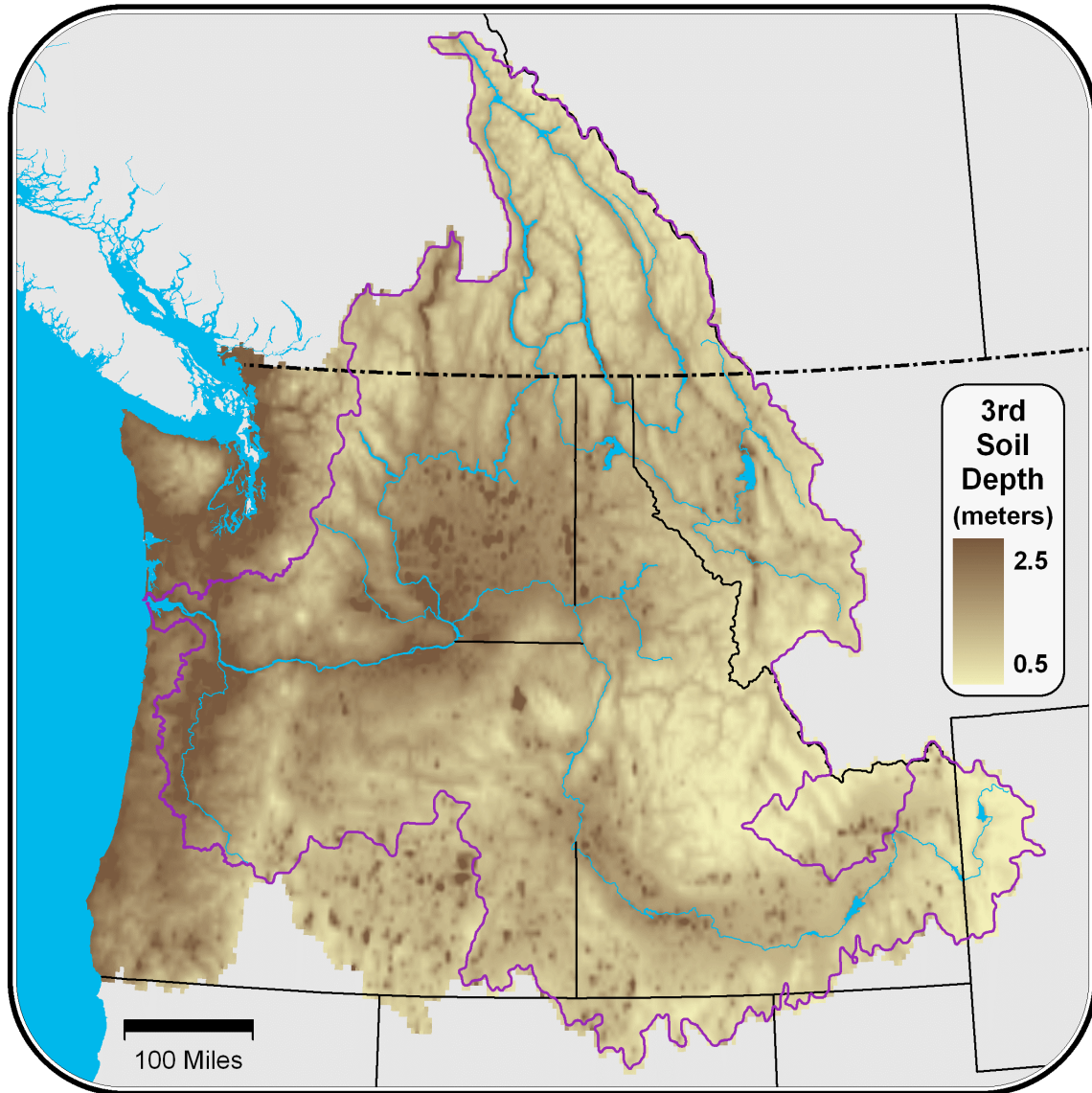
Figure 3 VIC model third (bottom) layer soil depths at 1/16^{\text{th}} degree latitude longitude resolution.
