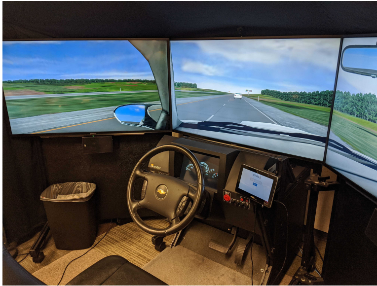
Figure 3.3: The NADS miniSim driving simulator setup used for data collection. The simulator is located on the University of Washington campus in Settle, WA.
