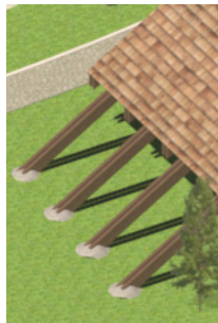
Figure 4.13 framing members extend from the roof to rock footings
