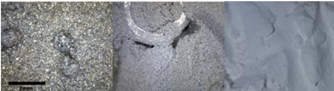
Figure 2.6: Propellants examined (from left to right) include JSC-1a, 30-micron aluminum powder, and 44-micron silica powder
