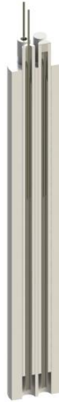
Figure 3.3: A cross-section of the double Langmuir probe and null probe used to probe the PPT. The needle configuration permitted convenient swapping of contaminated probe tips.
