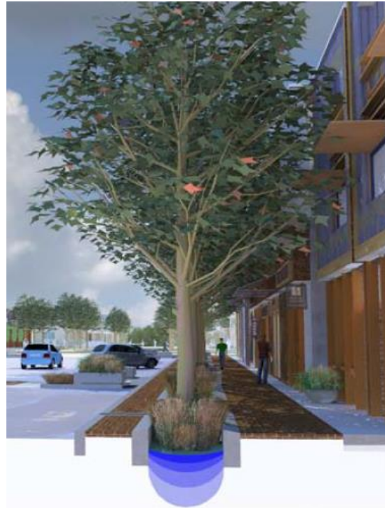
Figure 19. City of Greensburg, Kansas, Green stormwater infrastructure
