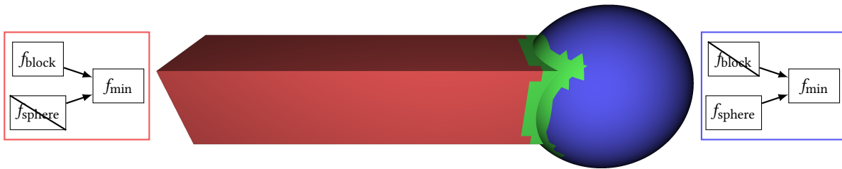
Figure 2.3: A rendering of an F-Rep model with shading based on a color-coding of pruned function composition trees. Each color represents a unique pruned tree configuration assigned to a leaf node of the sparse volume structure used to store the model. There are a total of three pruned tree permutations: f_{\text{sphere}} pruned (red), f_{\text{block}} pruned (blue), and no pruning (green). f_{\text{block}} and f_{\text{sphere}} each represent an operation grouping containing the defining functions for the block and sphere respectively, while f_{\text{min}} defines the union operation via the min function.
