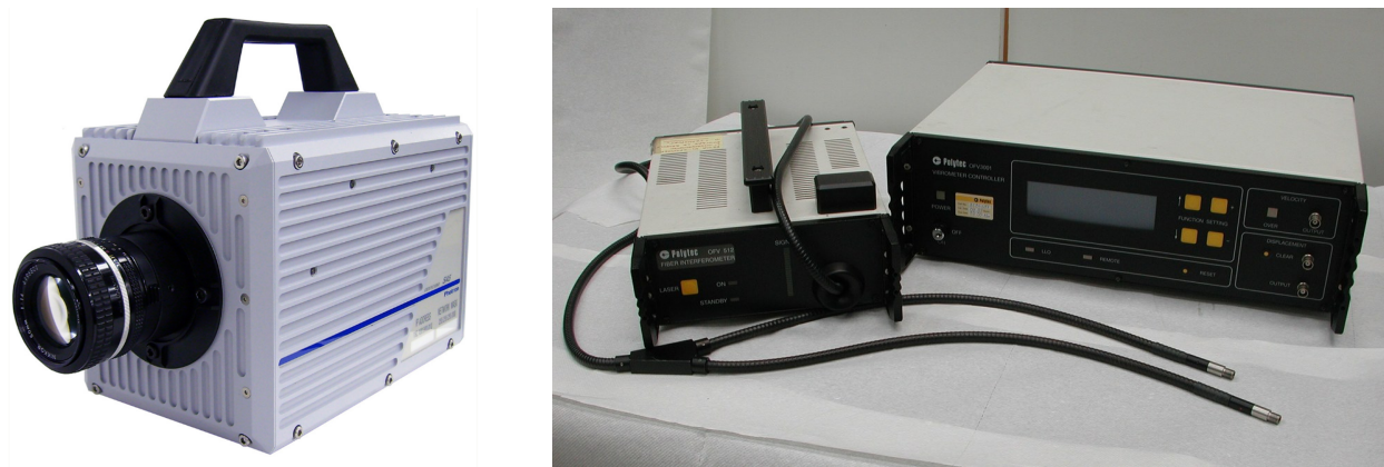
(a) DIC camera: Photron FASTCAM SA5.
