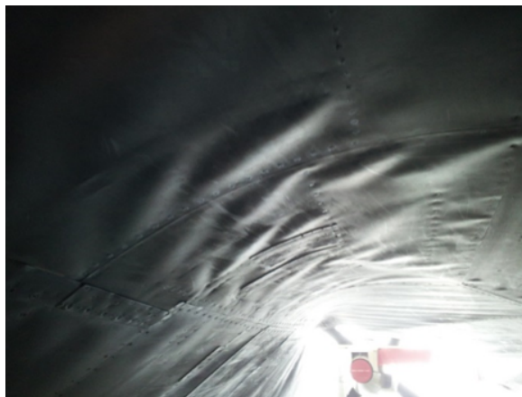
(b) Permanently buckled surface panel on the underside of the wing of a SR-71 Blackbird (photo courtesy of the United States Air Force).
