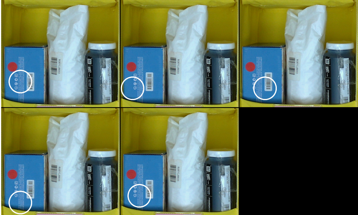
Figure 4.3: Second prompt: Annotate grasp points, refining the grasp points by shifting the suction cup projections in four neighboring directions
