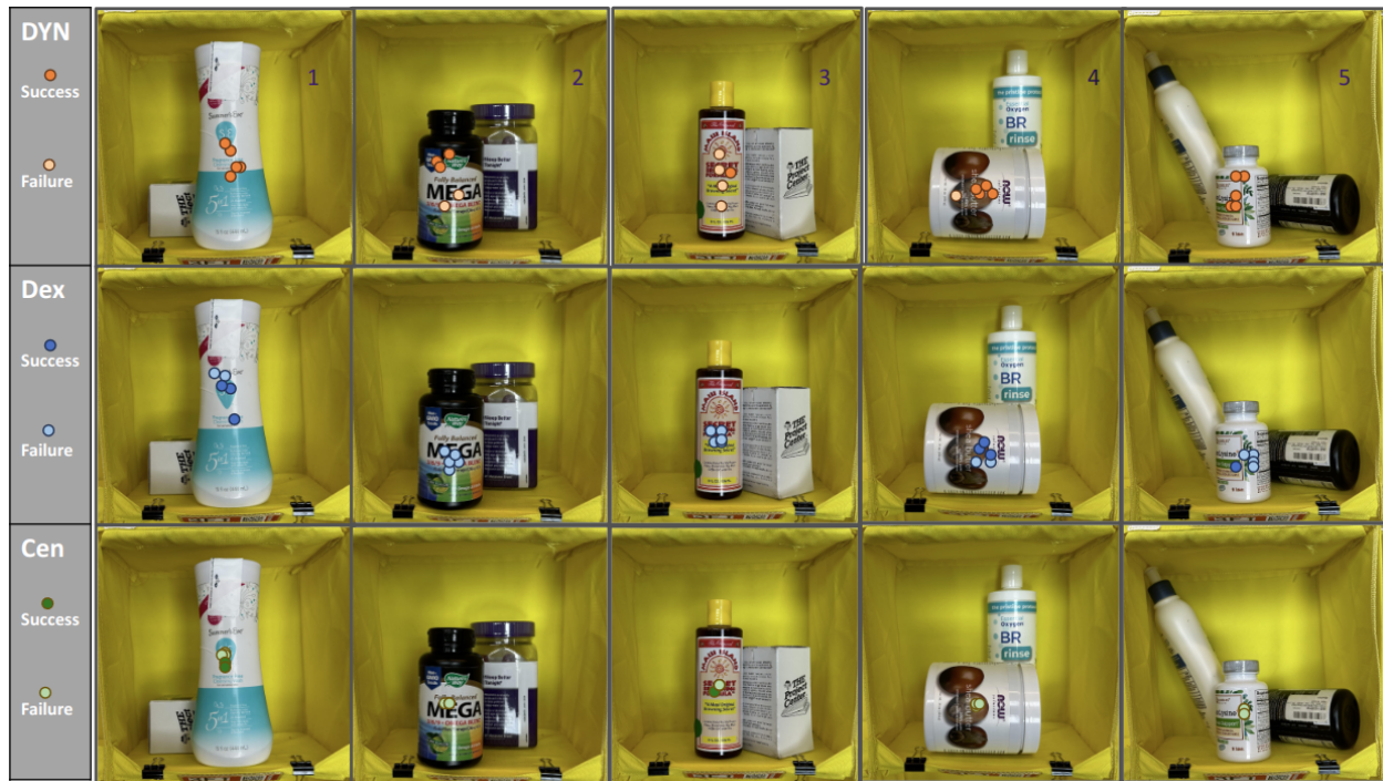
Figure 3.6: Real-world adversarial evaluation with five grasp points for each configuration: DYNAMO GRASP (our method), DexNet, and Centroid. The color-coded points represent the suggested grasp points success and failure from various algorithms. The successfully identified grasp points are marked by the color along the label “success” and “failure”.
