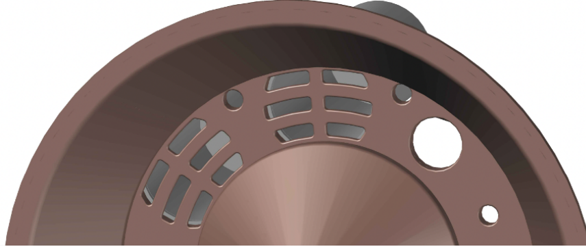
Figure 2.1: Louvers on HIT-SI3, dividing the confinement volume (copper) from the pumping volumes (gray).
