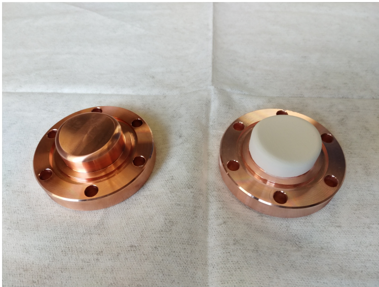
Figure 4.6: Two of the plugs used in place of pre-ionization sources, before and after the alumina coating was applied.
