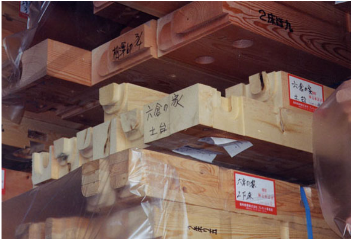
Photo 7.8. Yellow cedar dodai as a component of a pre-cut housing package.
