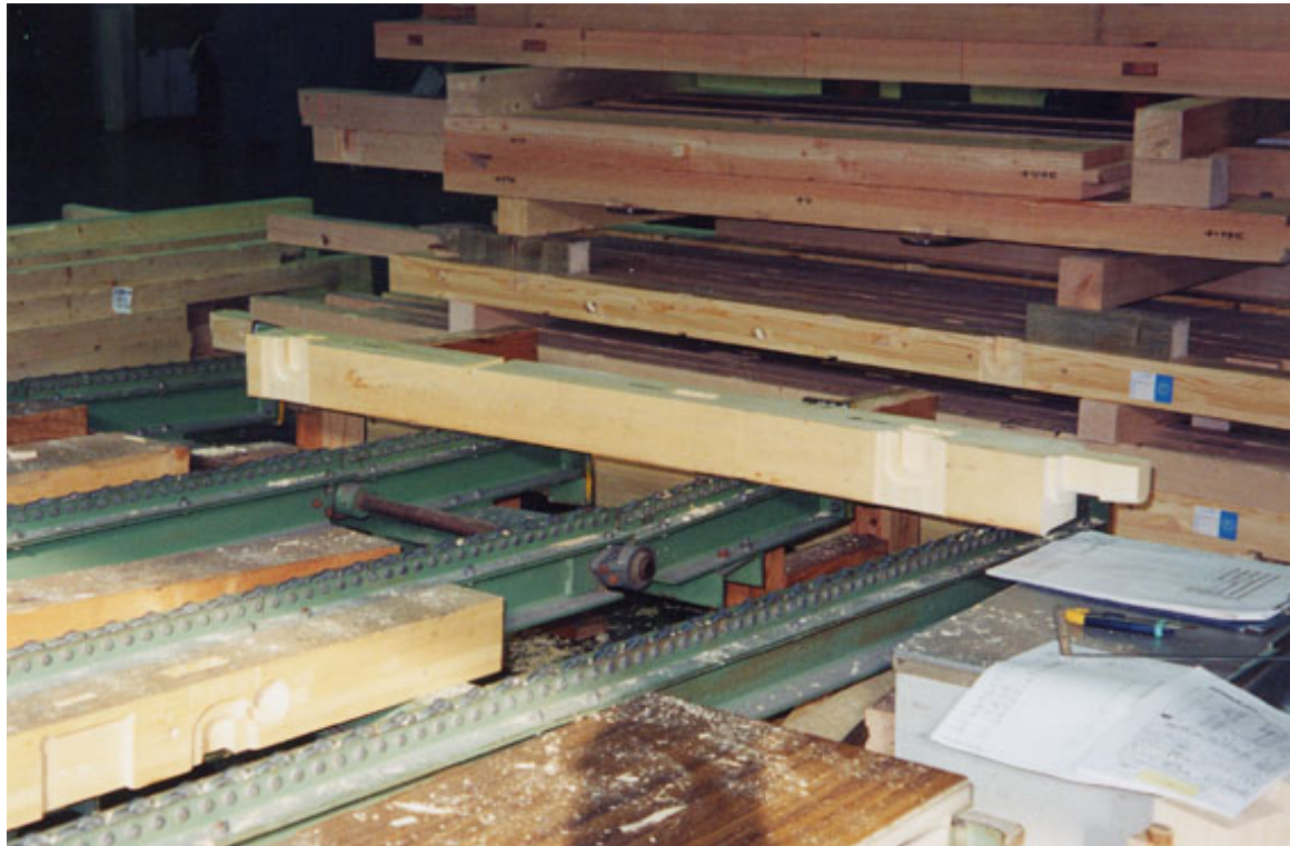
Photo 7.6. Yellow cedar dodai following machining process.
