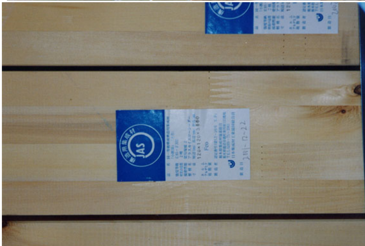
Photo 7.12. Alaska yellow cedar glu-lam beams prior to entering the hot press.
