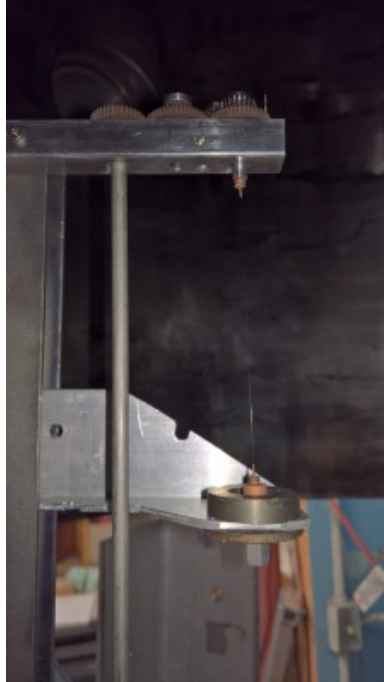
Figure 8.1: A photograph of the top of the pendulum stand showing the phi-top assembly, swing damper, pre-hanger, upper slug, and the upper clamping screw of the main fiber.
