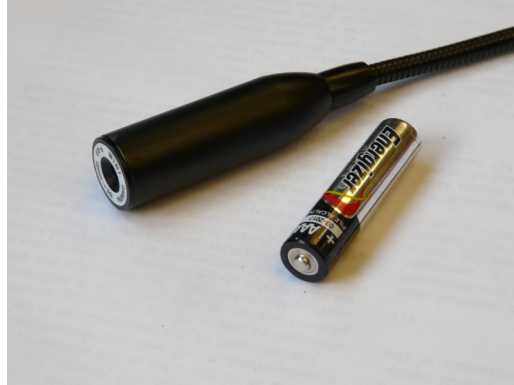
Figure 8.4: A photograph of the USB camera that was placed inside a vacuum nipple to create a low-cost vacuum compatible camera. An AAA battery is shown for scale.
