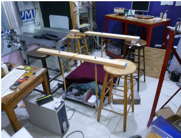
Figure 5.4: The setup used to isolate the iQuAC demonstrator from seismic and acoustic noise sources.
