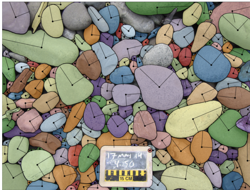
Figure 4.7: Example SegmentEveryGrain output for an ideal image from the Elwha River dataset.
