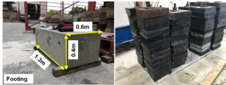
Figure 6.14: Model footing prior to placement and steel weights to replicate target contact pressure (from Motamed et al. (2020)).
