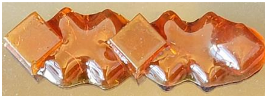
Figure C31. 15-BVIM gels, which contain solely dynamic crosslinks, experienced loss of fidelity during heating at 60 °C.
