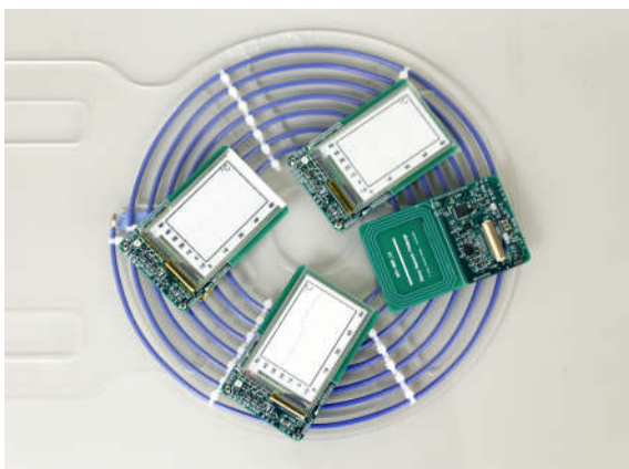
Figure 3.10: Image of four NFC-WISP placed on a magnetically coupled resonant charging coil.
