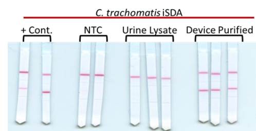
Figure 86. In-membrane NAAT comparing purified and non-purified samples. Input C. trachomatis concentration was \sim 10^4 copies per reaction.
