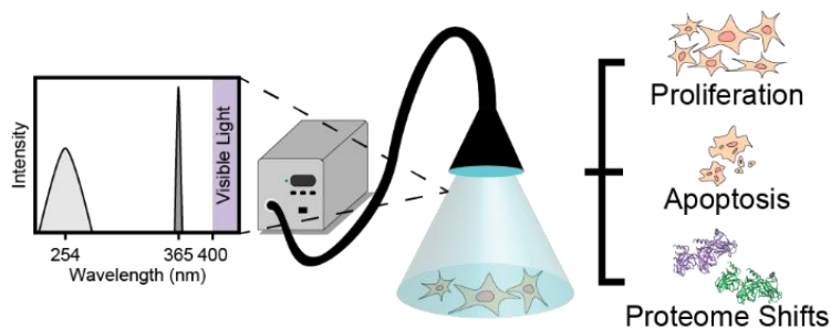
Figure 3.1. Cellular response to varying doses of 365 and 254 nm ultraviolet light was determined through quantitative analysis of cell proliferation, apoptotic events, and proteomic shifts.
