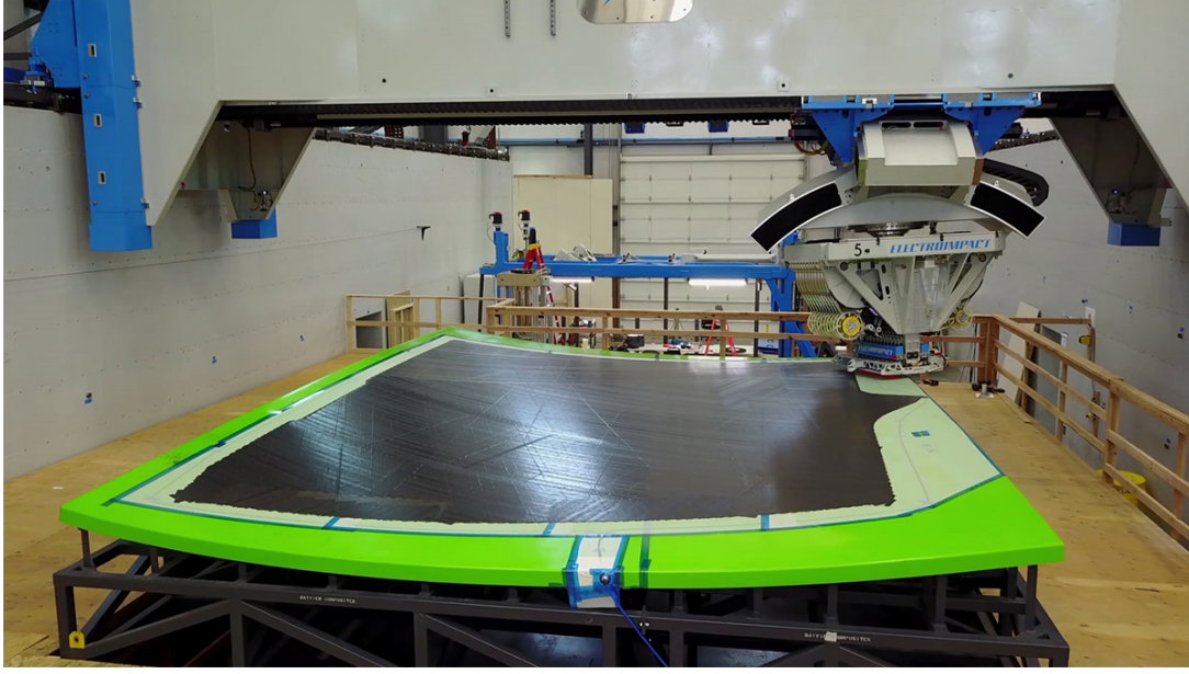
Figure 1.10: AFP system during operation [32].
