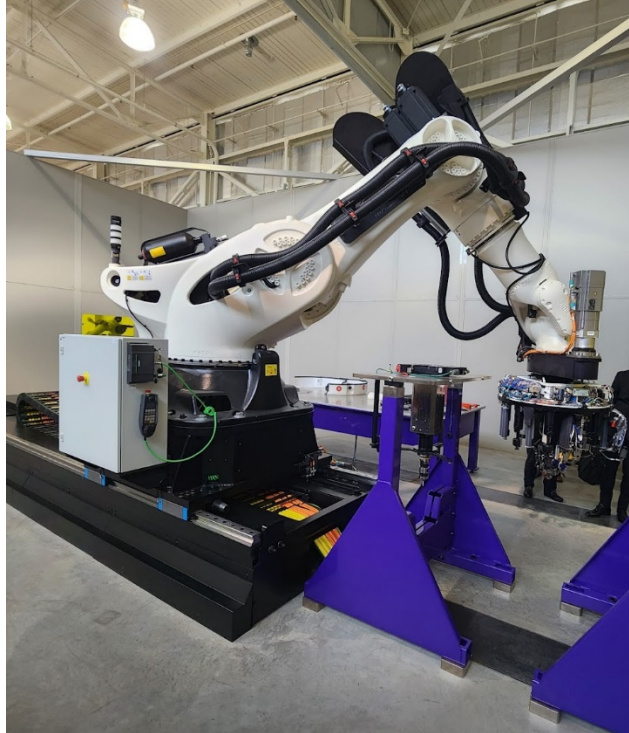
Figure 8. Example of a laser-assisted thermoplastic composite AFP.
